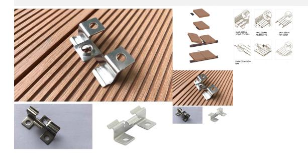
Concealed Hidden Stainless Steel T Clips Fixings for Composite Decking Boards - sold in bags of 100. Recommended 20 per sq m on every joist ie. 8 per board at 400mm joist centres.
